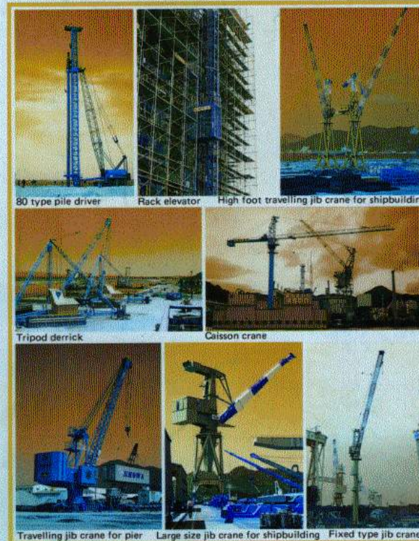
Travelling jib crane for pier Large size jib crane for shipbuilding Fixed type jib crane
